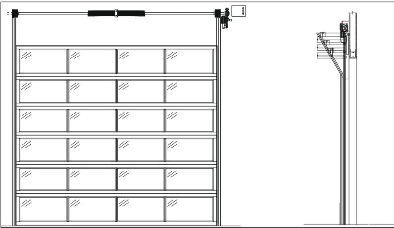
The Sovereign system is balanced by the use of torsion springs connected to a rotating shaft. The shaft ends are attached to cable drums that lift / lower the curtain, and no overhead tracks. This means no interfering with lights, HVAC, or sprinkler systems.
